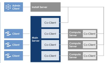
This picture shows a real configuration with interconnected Esprit-servers. The install server is used to keep the software of all involved systems automatically up to date.
